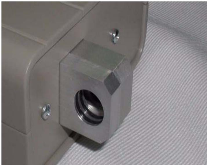
**FIGURE 2-2 Aluminum Block with Microphone Ports**
