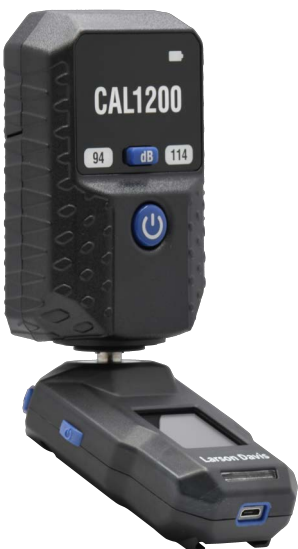
FIGURE 2-2 Dosimeter display during calibration
