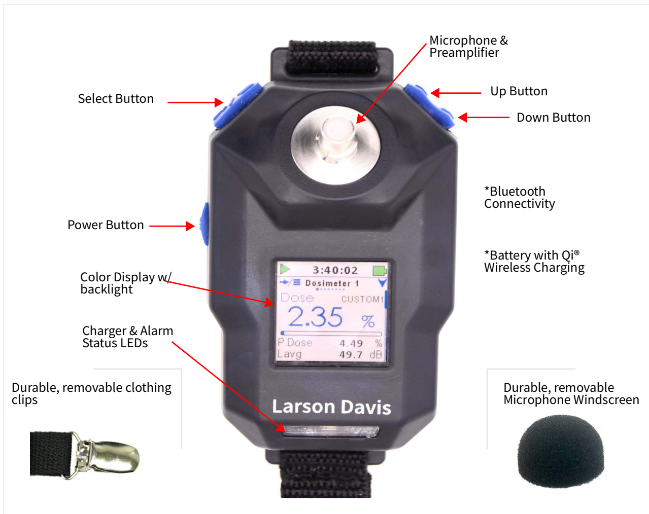
FIGURE 1-8 Components of the Spartan Model 730
