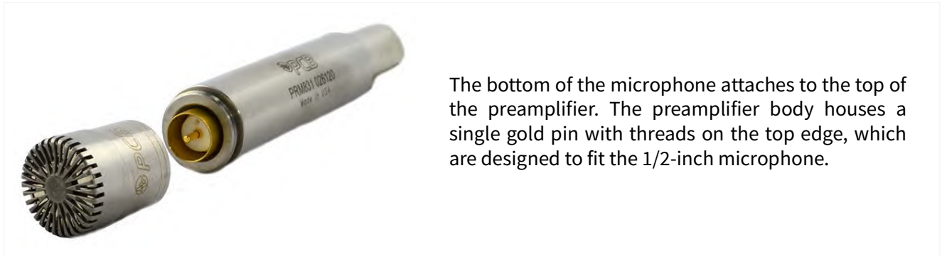
FIGURE 2-1 Microphone and Preamplifier PRM831
