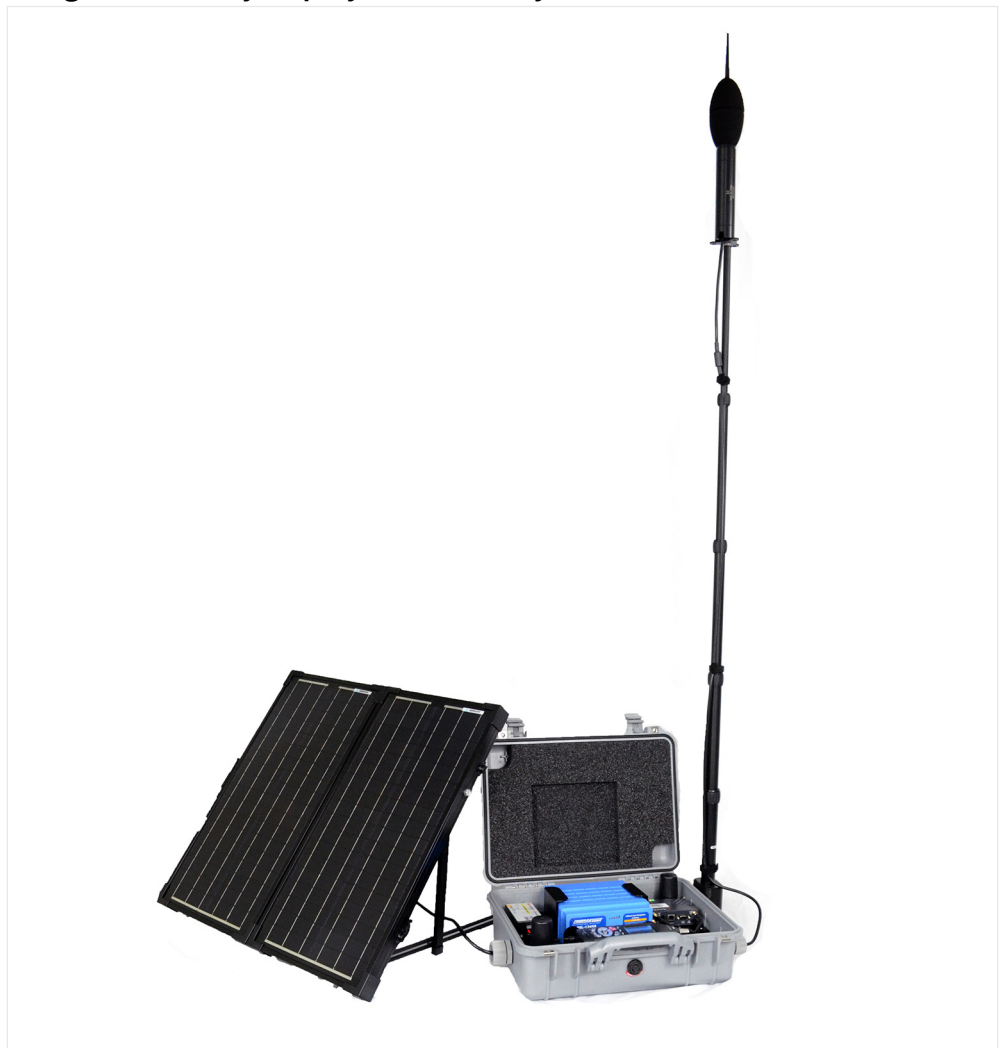
Figure 3-1 Fully-deployed NMS044 system
