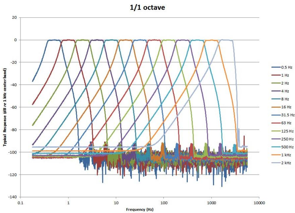
**FIGURE A-30 1/1 OBA 8.0 Hz Filter Response**
