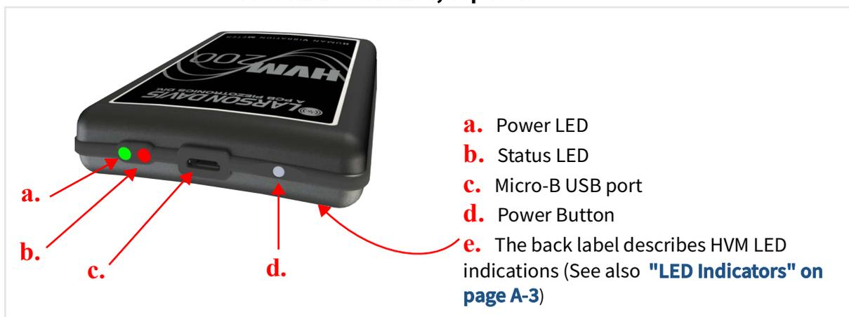
The power button is multi-functional, and provides each of the following functions:
