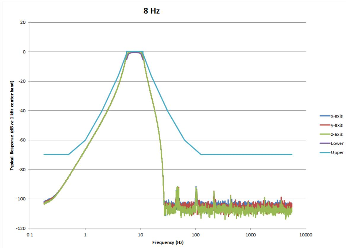
**FIGURE A-31 1/1 OBA 8.0 Hz Filter Response: Pass-band**
