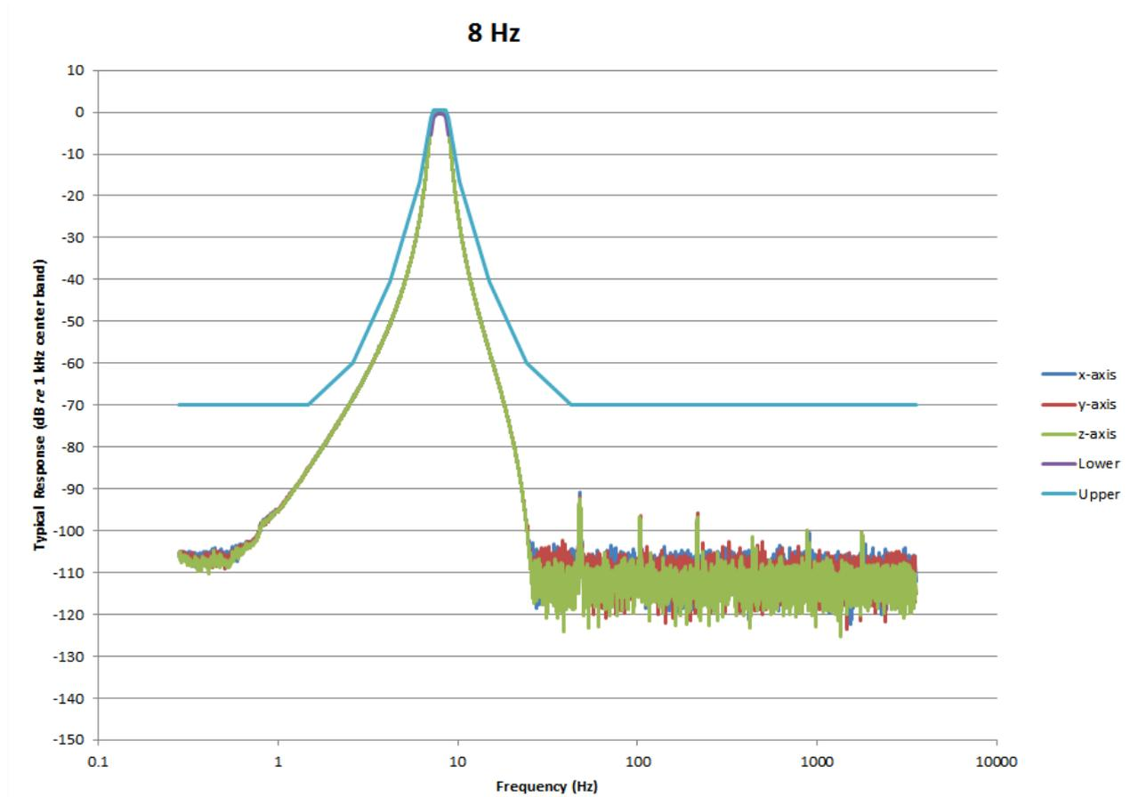
**FIGURE A-38 1/3 OBA 8.0 Hz Filter Response: Pass-band**
