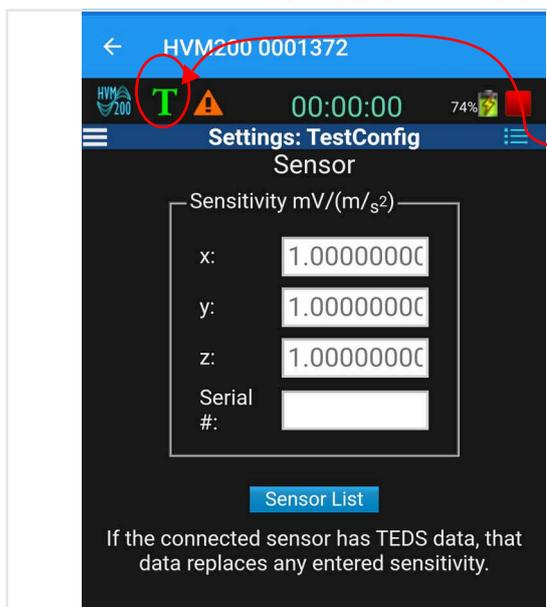
If you are using a sensor equipped with Transducer Electronic Data Sheet (TEDS), the **Teds (T) icon** appears in the top bar, and the model, serial number, and sensitivity details automatically display.
