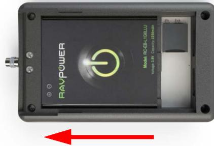
**Step 3.** Slide the back battery cover onto the HVM200.
