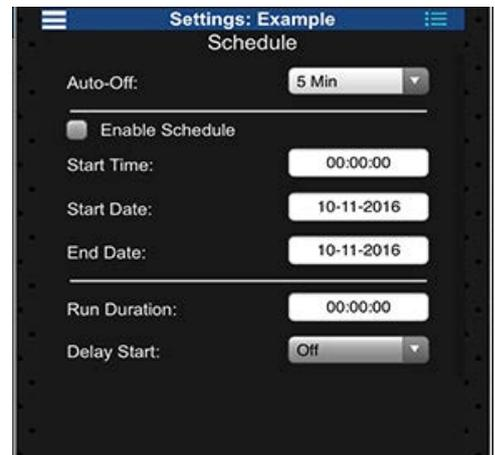
**Step 3.** Select the checkbox in-line with **Enable Schedule**.
