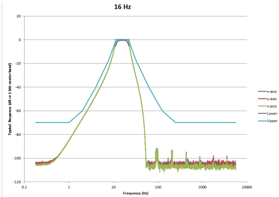
**FIGURE A-33 1/1 OBA 16.0 Hz Filter Response: Pass-band**
