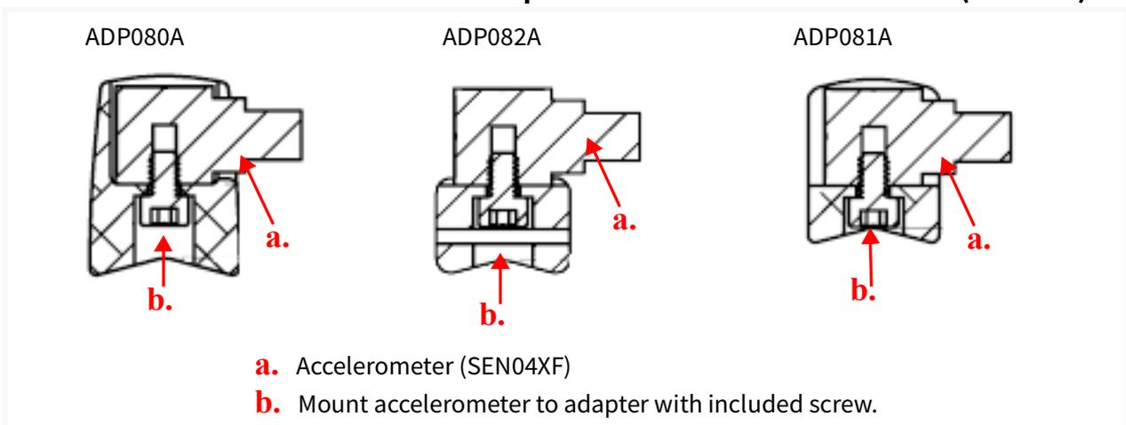
**Step 2.** Connect the accelerometer and cable as shown in *Figure 3-1*.
