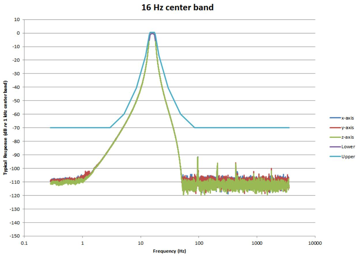
**FIGURE A-40 1/3 OBA 16.0 Hz Filter Response: Pass-band**
