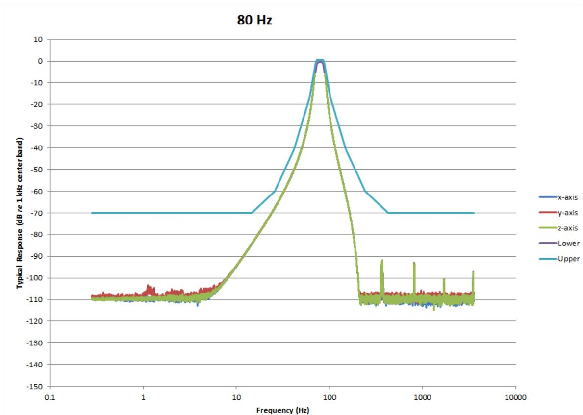
FIGURE A-42 1/3 OBA 80.0 Hz Passband Filter Response
