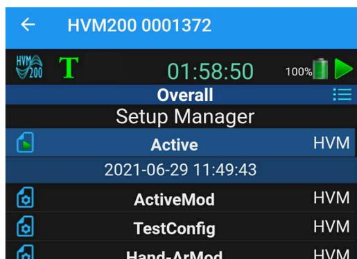
**Step 2.** Tap and hold the name of the Setup you want to use for the next measurement, then tap **Set as Active** in the menu that appears.
