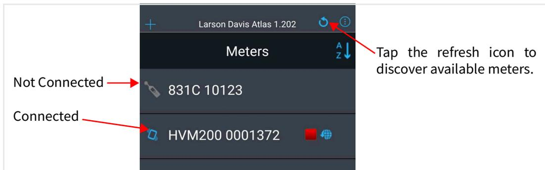
**Step 4.** Tap to select the “HVM <serial number>.” This opens the meter interface in the app.
