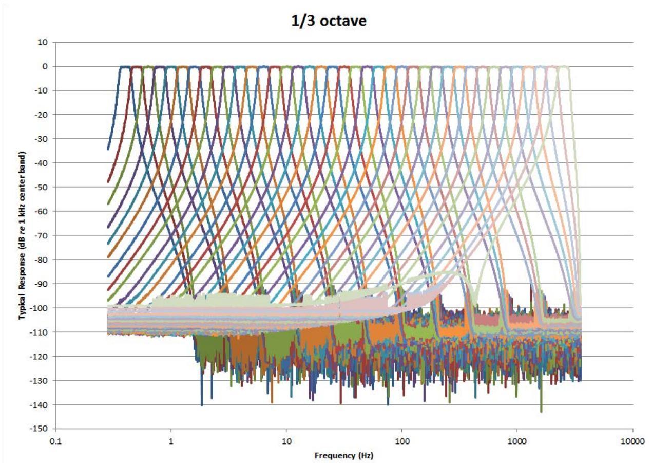
**FIGURE A-35 1/3 OBA 0.4 Hz Filter Response**
