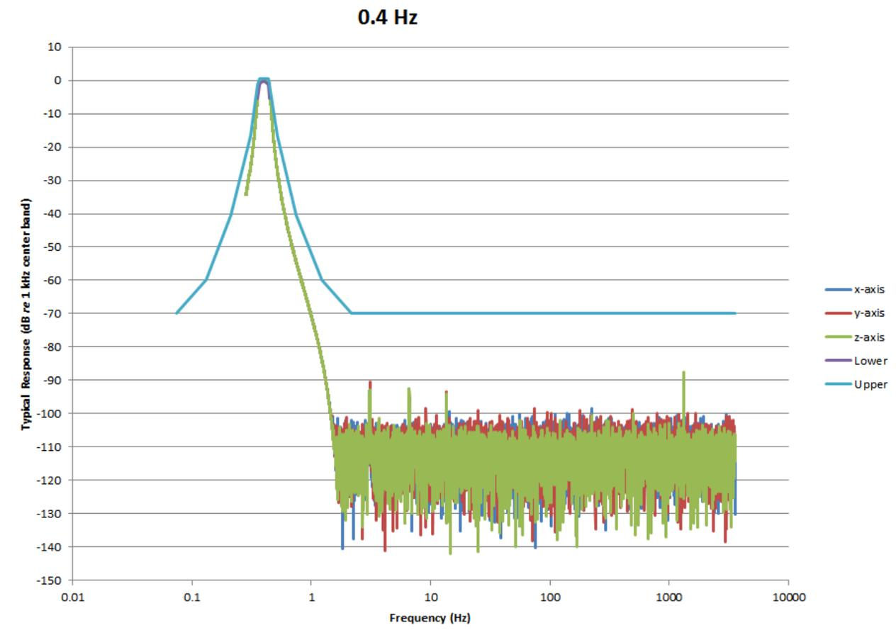
FIGURE A-36 1/3 OBA 0.4 Hz Filter Response: Pass-band
