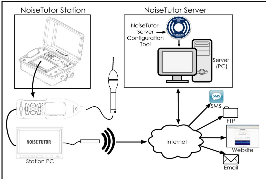
**FIGURE 1-1 Components and Architecture - NoiseTutor System**
