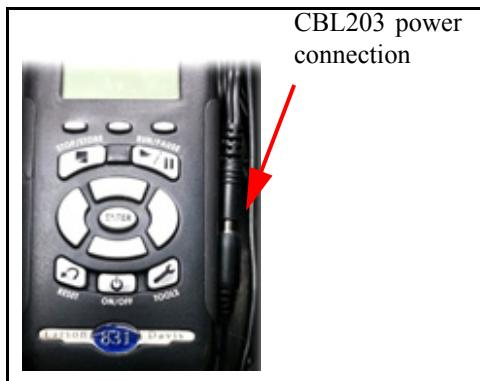
**FIGURE C-6 Connected Power**
