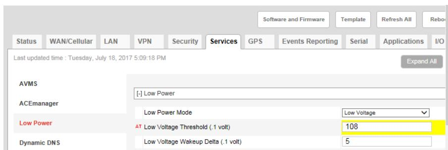
**FIGURE C-22 Shutoff Voltage for LS300**
