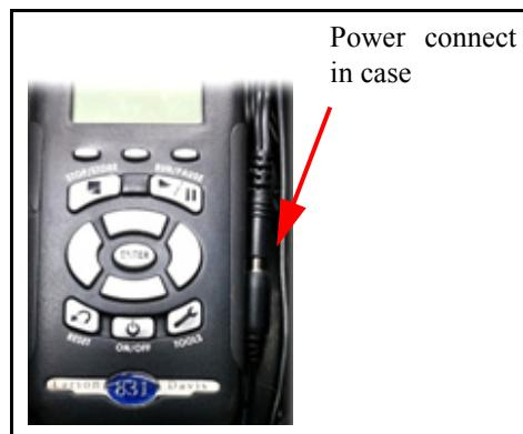
**FIGURE C-13 Connected Power**
