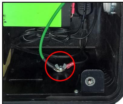
**FIGURE C-7 Connected Ground**
