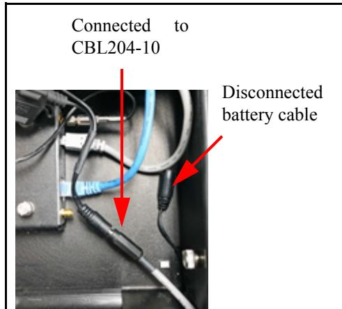
**FIGURE C-18 CBL204-10 Connected to NoiseTutor**
