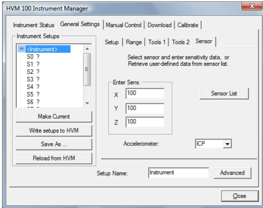
In addition to displaying the accelerometer type and its sensitivity, the Sensor Tab page permits access to a transducer database in the form of a sensor list from which a user can select a sensor, add/edit a sensor, delete a sensor or
