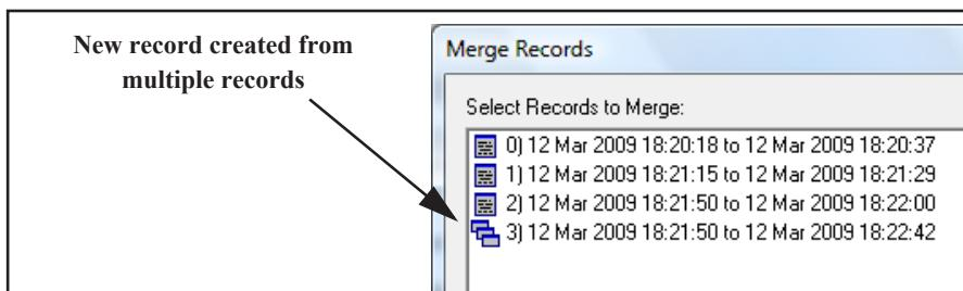
Press **Done** to close the Merge Records dialog box. To display the new record, open the records pull-down list at the top of the Data Record window, highlight the merged record and click with the left mouse button.
