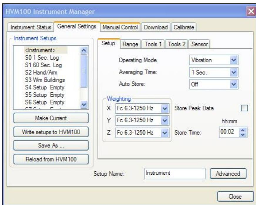
When the connection has been successfully completed, the names of the Instrument Setups stored in these registers are listed on the left of the screen under the heading "Instrument Setups", beginning with the active setup named <Instrument>. Setup information displayed corresponds to the setup which was active at the time of connection.
