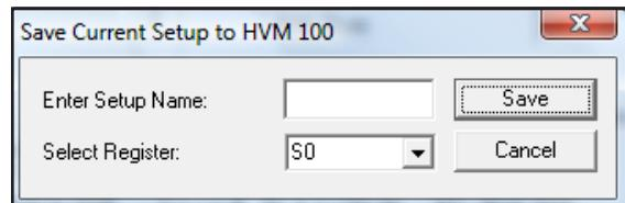
Type in a Setup Name and select an HVM100 register into which to store the setup. The information is immediately updated in the HVM and in Blaze instrument manager.
