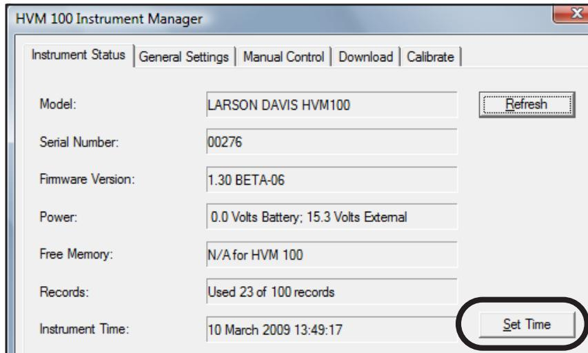
*“Synchronize to computer time,” forces the active HVM100’s internal clock to match that of the connected computer.*
