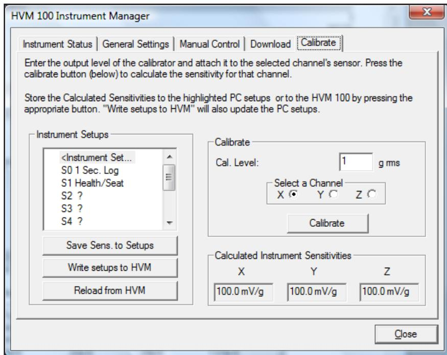
The sensitivity values displayed on the right side of the screen are either values entered at the time the setup was created or values determined as a result of a previous calibration.
