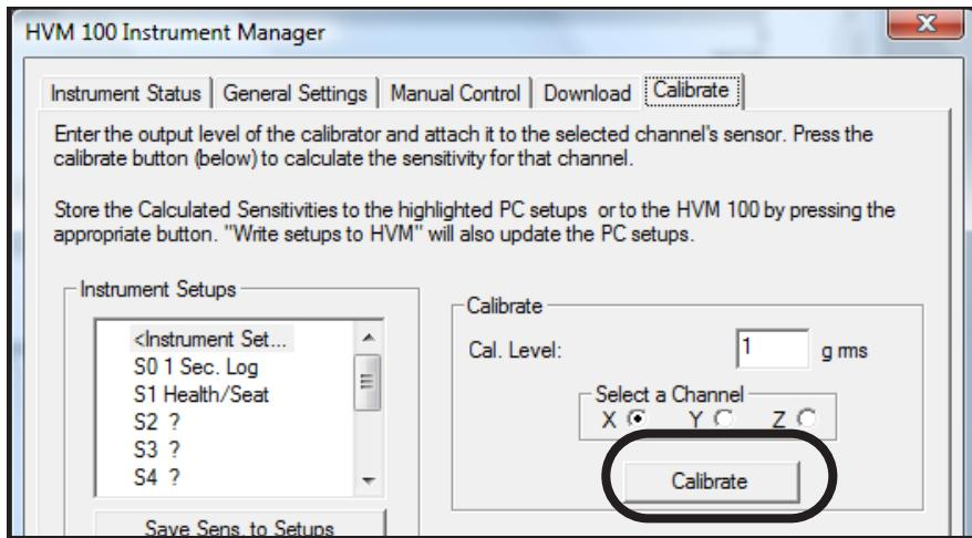
Prompts will appear on the screen asking you to confirm that the calibration data may be reset and that the accelerometer is properly connected and that the calibrator is operating. A response of **No** to either of these prompts will abort the calibration process. The calibration process will continue if both prompts are answered **Yes**.
