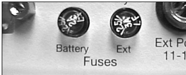
**Step 3** Replace defective fuse with a new fuse
