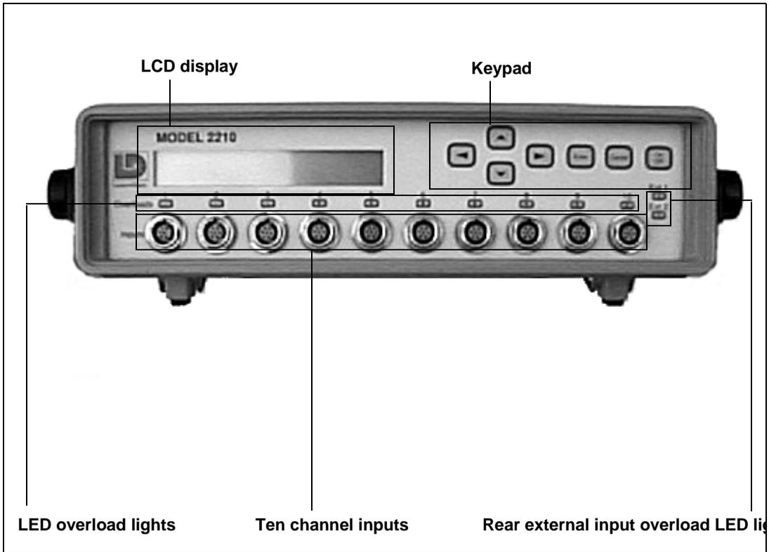
Figure 2-1 Model 2210 Front Panel.
