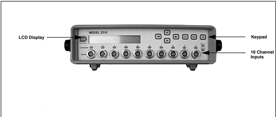
Figure 1-1 *Model 2210*. The Model 2210 is a flexible microphone signal conditioner/multiplexer with manual and remote capabilities.
