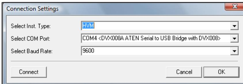
From the Connection Settings dialog box, select HVM100 as the instrument type, the computer Com Port to which the instrument is connected and the desired Baud Rate.
