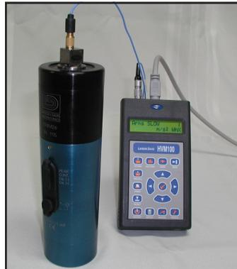
**Step 4** Press **Calibrate** to initiate the calibration process.
