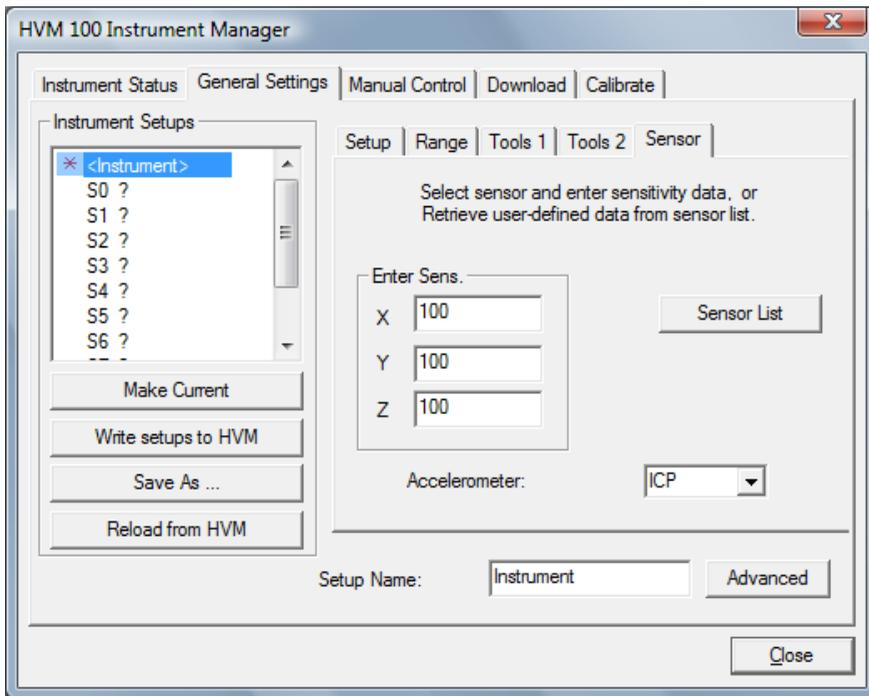
In addition to displaying the accelerometer type and its sensitivity, the Sensor Tab page permits access to a transducer database in the form of a sensor list from which a user can select a sensor, add/edit a sensor, delete a sensor or
