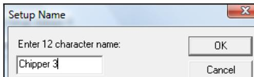
Type in a name for this setup and press **OK**. This feature permits a user to create a Database Setup without having to first store it to the HVM100. However, the user does have to have an HVM100 connected to be able to perform this operation.
