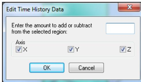
Enter a numerical value and select to which axis, or axes, the modification is to be applied and click OK
