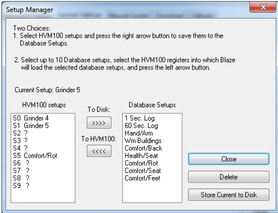
The nine Database Setups listed above are default setups provided with the software which cannot be deleted. The user may create and store new setups which will be added to these default setups, but the list will always contain these nine as a minimum.
