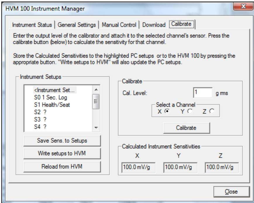
The sensitivity values displayed on the right side of the screen are either values entered at the time the setup was created or values determined as a result of a previous calibration.
