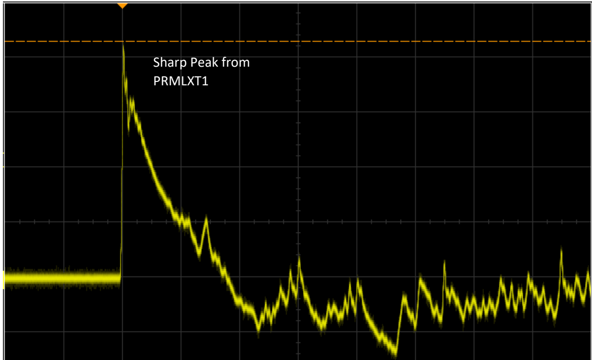
Figure 1 - Oscilloscope waveform from 377C10/PRMLXT1
