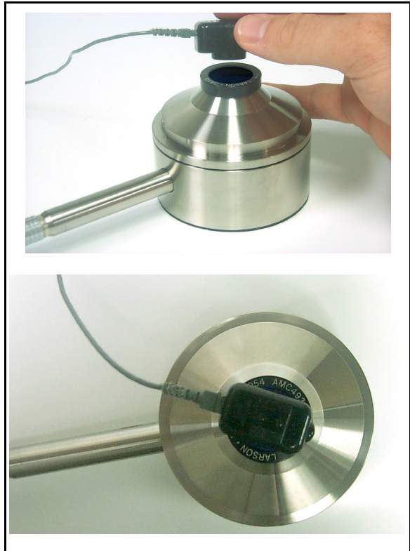
FIGURE 5-41 Vibrator being placed and centered on mastoid
