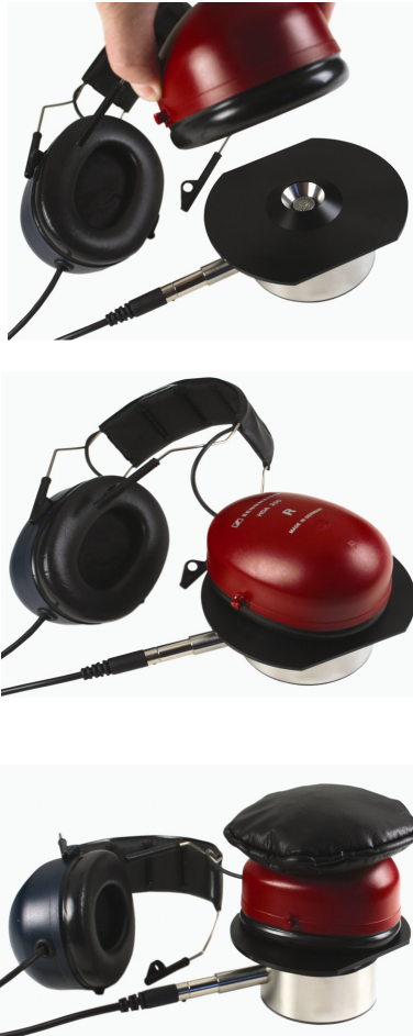
FIGURE 5-39 Sennheiser earphone and weight bag being installed on AEC201
