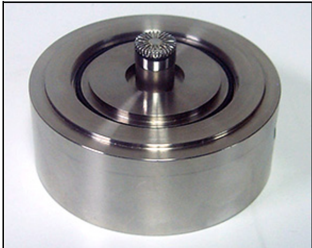
FIGURE 5-28 Microphone installed on AEC201
