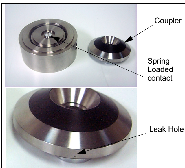
FIGURE 5-27 AEC201 with coupler, leak hole
