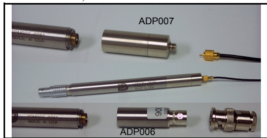
FIGURE 5-46 Adapters to connect to B & K ® mastoid
