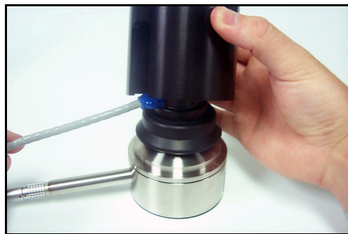
FIGURE 5-25 Retainer Ring being installed over headphone.
