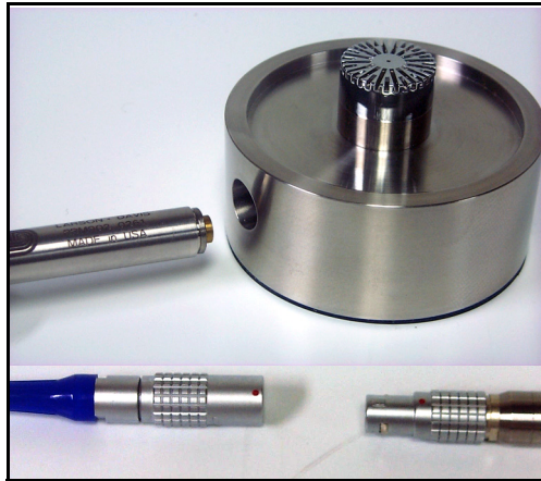
FIGURE 5-19 Preamp connecting to AEC100 and Extension Cable
