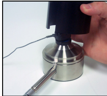
FIGURE 5-43 Retainer Ring being placed over vibrator
