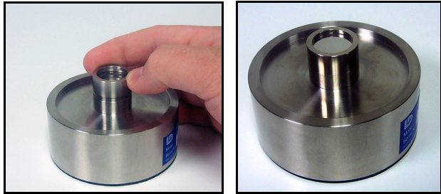
FIGURE 5-23 Installing Protective Ring on 2575 Microphone
