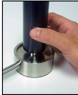
FIGURE 5-21 Starting Calibration tone with on switch
