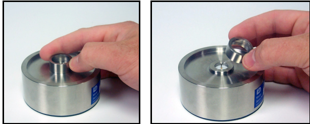
FIGURE 5-17 Protective ring being removed from AEC100
