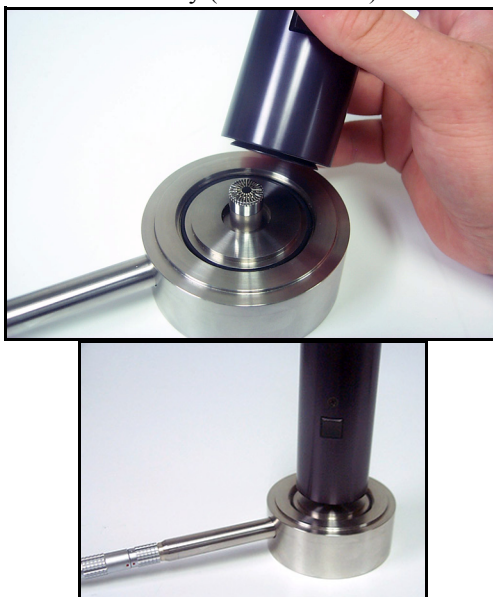
FIGURE 5-30 Installing the CAL250 on AEC201
