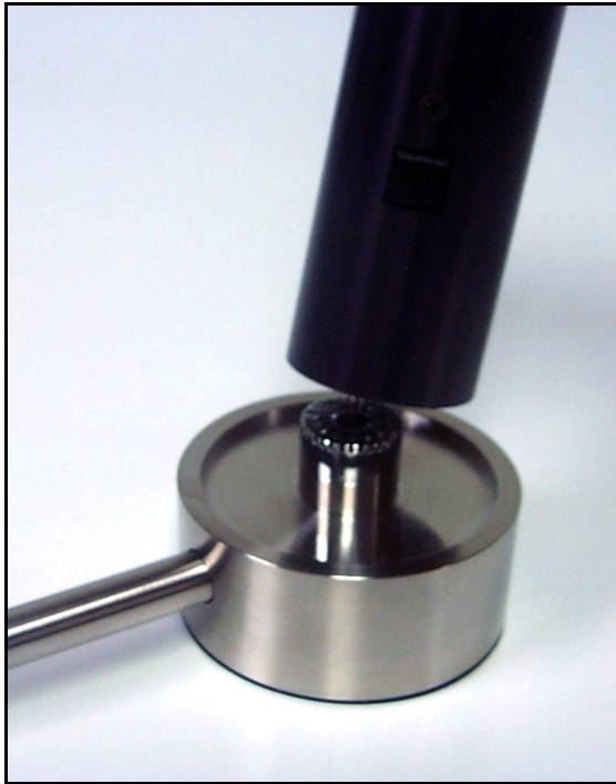
FIGURE 5-20 CAL250 being lowered onto 2575 microphone
