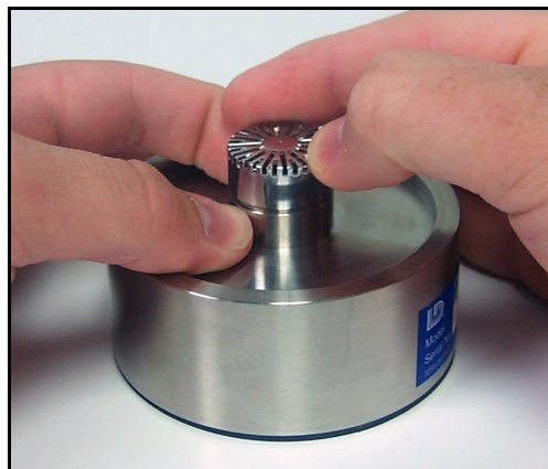
FIGURE 5-22 Removing grid cap from 2575 Microphone
