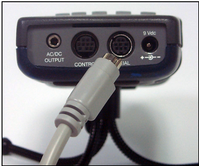
FIGURE 5-13 Connecting CBL006 to 824
