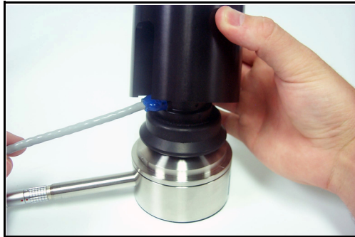
FIGURE 5-34 Retainer ring being installed on AEC201
