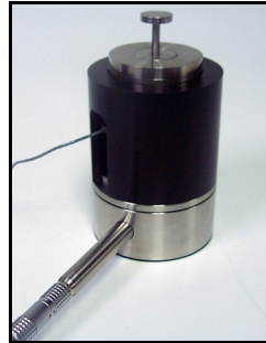
FIGURE 5-44 Artificial ear with vibrator and mass installed
