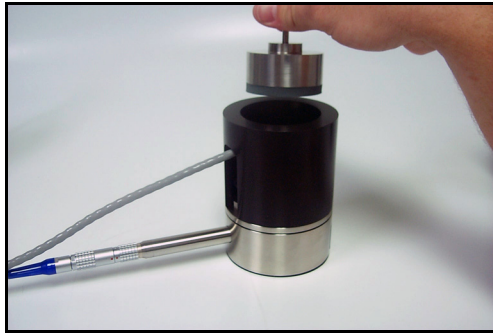
FIGURE 5-26 Mass being installed on AEC100.
