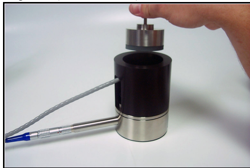
FIGURE 5-35 Mass being lowered onto headphone
