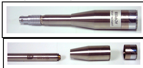
FIGURE 5-45 ADP008 being installed on PRM902
