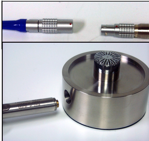
FIGURE 5-15 Preamp connecting to extension cable and to AEC100
